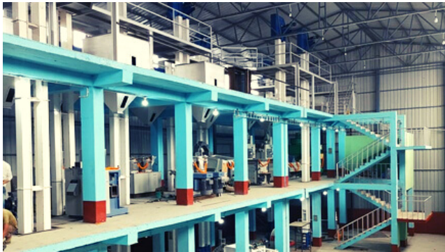
8 TPH Capacity Rice Milling Plant for Parboiled Rice
